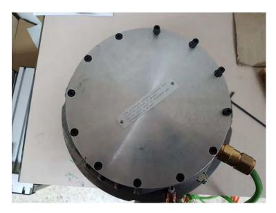
2.- Connect the cables in position, power cables on the ceramic connection block , signal cables on the green plastic connector
