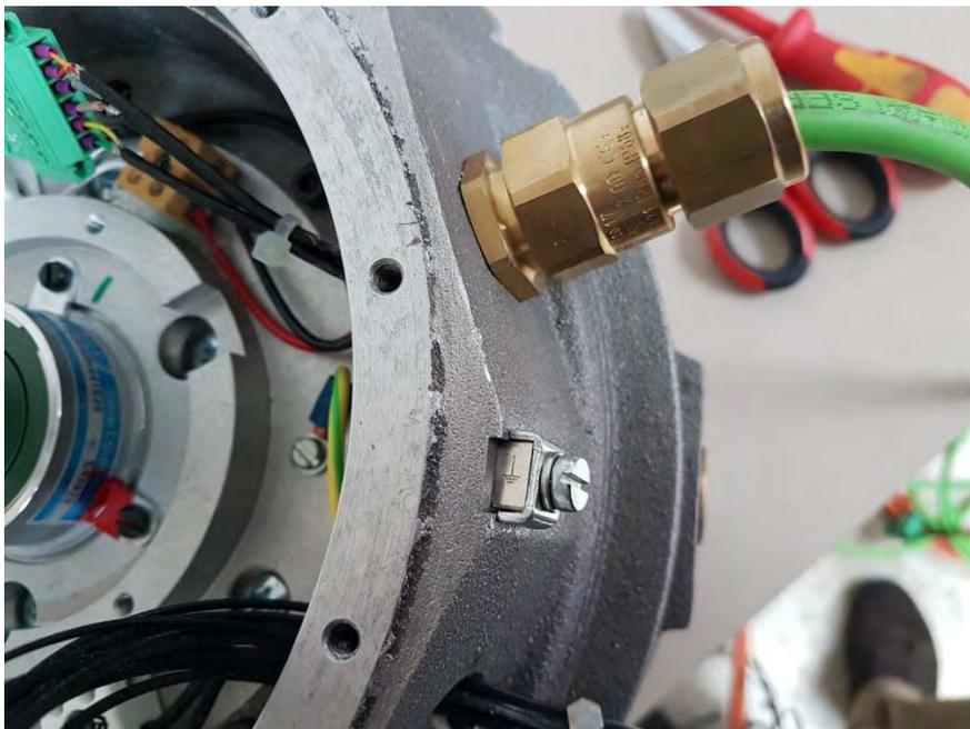
The cable gland shall be ATEX / IECEx certified, as appropriate, with “db” type off protection, suitable for the condition of use, installed correctly and must have a minimum thread length of 8mm. Use cable gland with some kind of shielding fixing system to avoid EMC problems, the use of conduit component is not allowed
