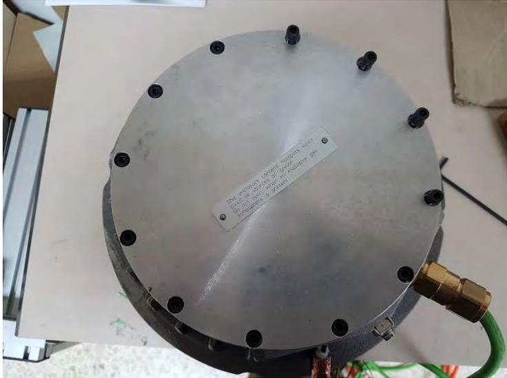
2.- Connect the cables in position, power cables on the ceramic connection block , signal cables on the green plastic connector
