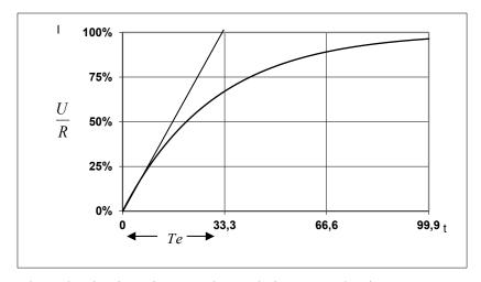
The value is given in ms when L is in mH and R in  $\Omega$
